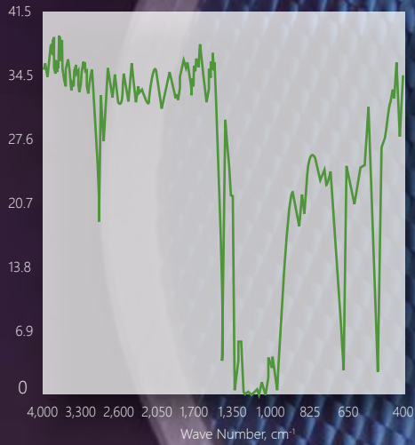
Infrared Scan of Everflon™ ETFE
