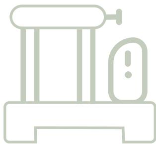
Ram extrusion is a way of manufacturing continuous length of rods, tubes or profile by feeding successive charges of PTFE powder to a die tube, where a reciprocating ram compacts the powder. Subsequent charges are then compressed onto each other and forced by the ram through the die tube that is heated above the melting point of PTFE, where the PTFE particles and the individual charges are sintered together.
